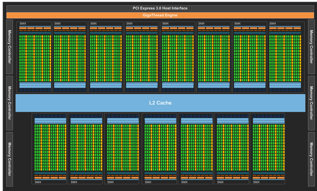
Figure 2.4: Schematic representation of the NVidia Kepler architecture (obtained from [1]).
